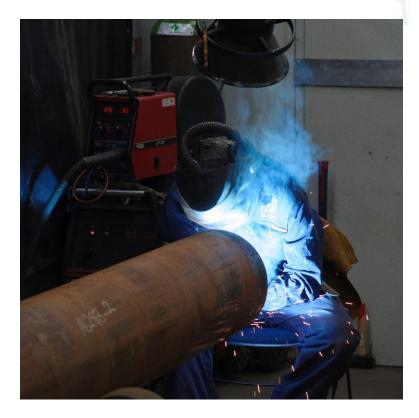
Where flexible arm fume extraction is used, the position of the extraction hood is crucial! If too far away, it has no benefit; it usually needs to be within 30cm of the weld.
