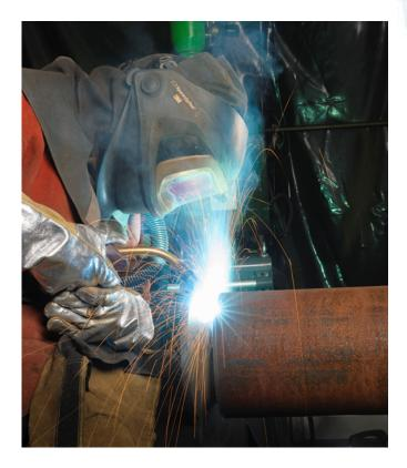
The welder is being exposed to welding fume and gases, which are not being properly controlled.
