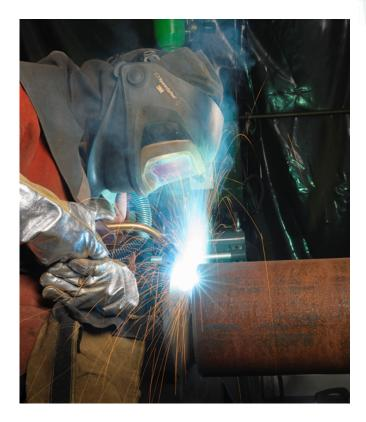
Welding fume contains a cocktail of airborne gases and very fine particles.
